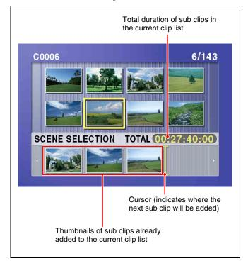
To move the cursor in the scene selection window After carrying out step 3 to display the scene selection window, press the  $\Leftrightarrow$  or  $\Rightarrow$  button.
